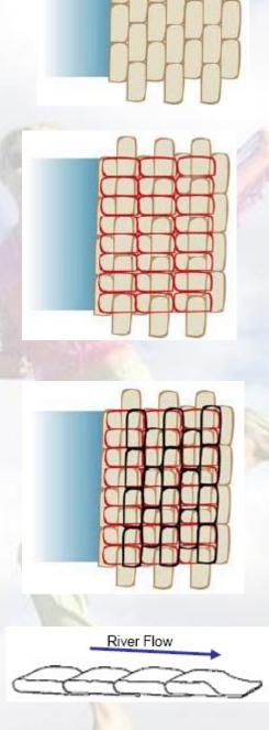
side of the dyke, producing a step-like appearance. Weave the polyethylene sheet between the courses of sandbags as to have at least two layers of sandbags protecting the polyethylene sheet from debris punctures. Maximum depth of the polyethylene sheet should
