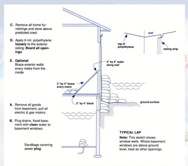
**Note:** This sketch describes a method of protecting an individual dwelling from flooding using polyethylene and sandbags. Although the method has been successful, constant surveillance and maintenance of the emergency flood barrier is a requirement during the duration of the flood. This method is **not** recommended where the predicted crest extends 1.3 metres over the water level in the basement.
